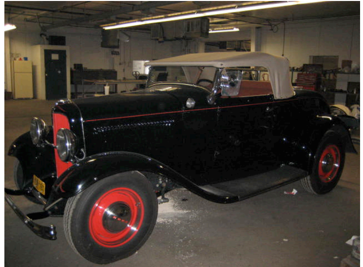
Dr. Skene's 32 Ford Roadster with finished new 3" chopped top with full polished stainless steel top iron and oak wood bows. Delphi 2010.
