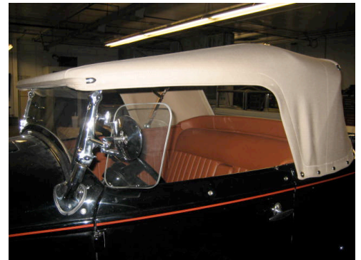
Dr. Skene's 32 Ford Roadster with finished new 3" chopped top with full polished stainless steel top iron and oak wood bows. Delphi 2010.
